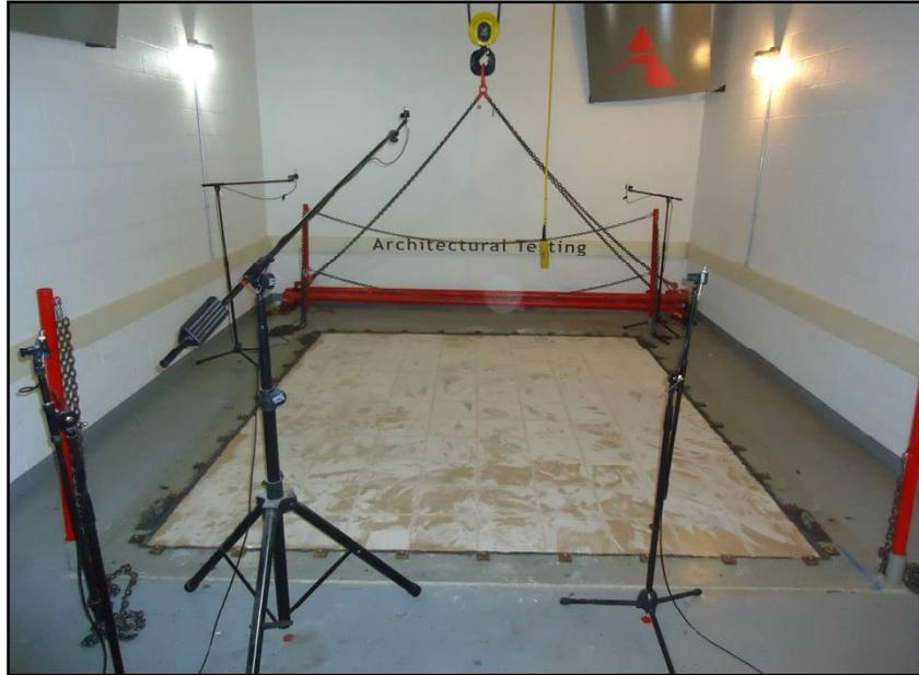
**Source Room View of Test Specimen Installation**
